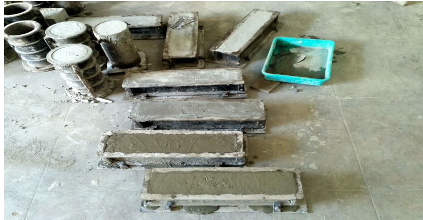
Fig. 4.2 casting of flexure beams
