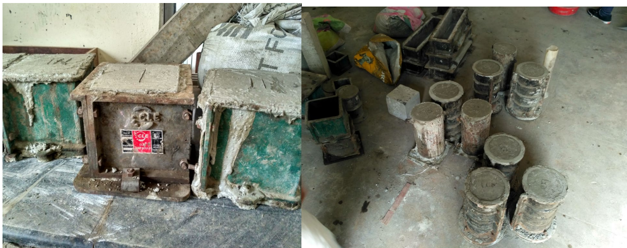
Fig. 4.1 Casting of Cubes and cylinders
