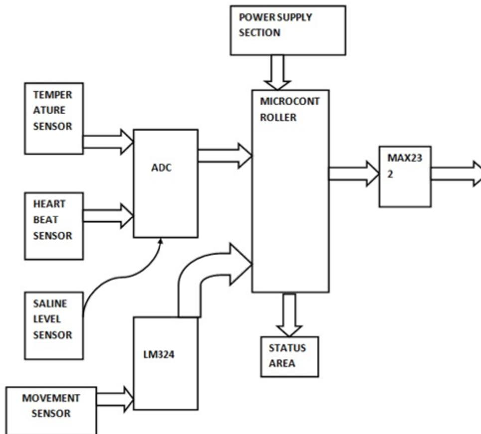
Figure 1: block diagram
