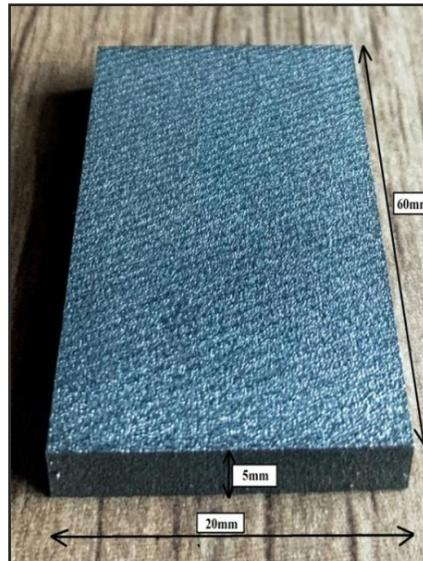
**Fig. 2.** Photograph of fabricated selective laser melted 316L stainless steel specimen of 5 mm thickness formed using recommended process parameters.
