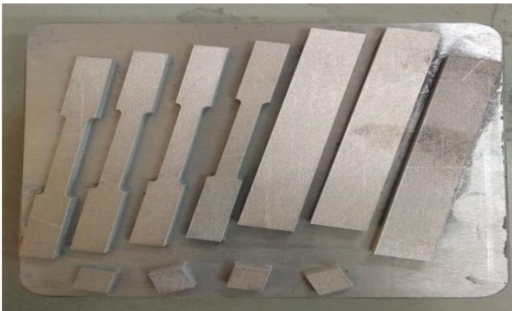
Fig. 3 Sample in as-fabricated state on the substrate plate
