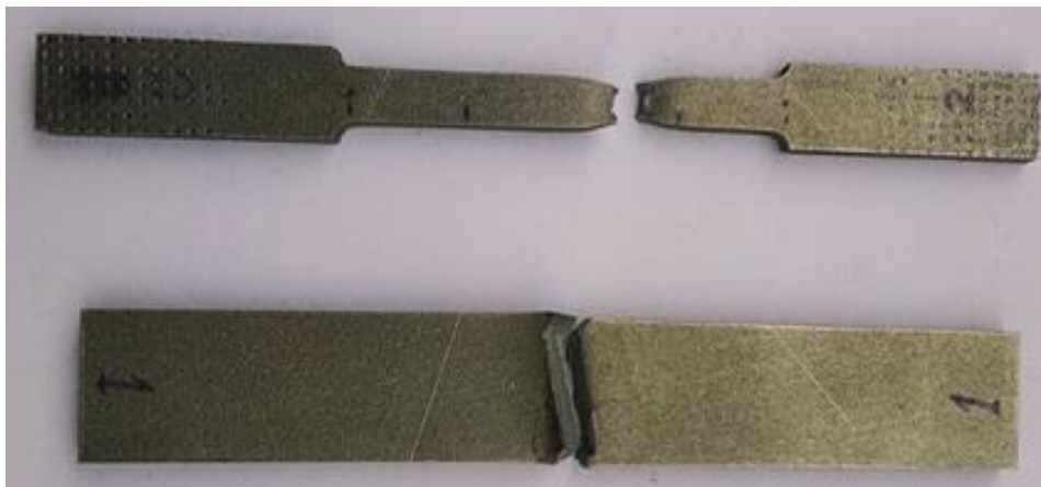
Fig. 6 Fractured Samples of Tensile and Bending Specimen
