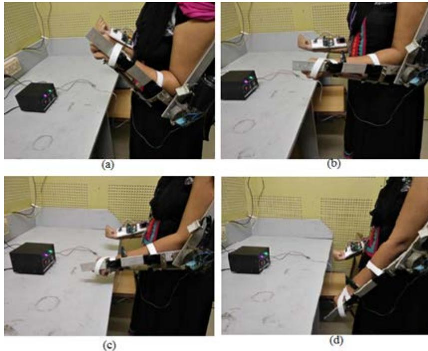
**Figure 7.**Photograph of upper limb exoskeleton at various angle
