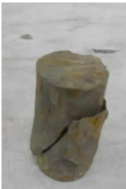
Figure 5 : Failure of a specimen by shearing
