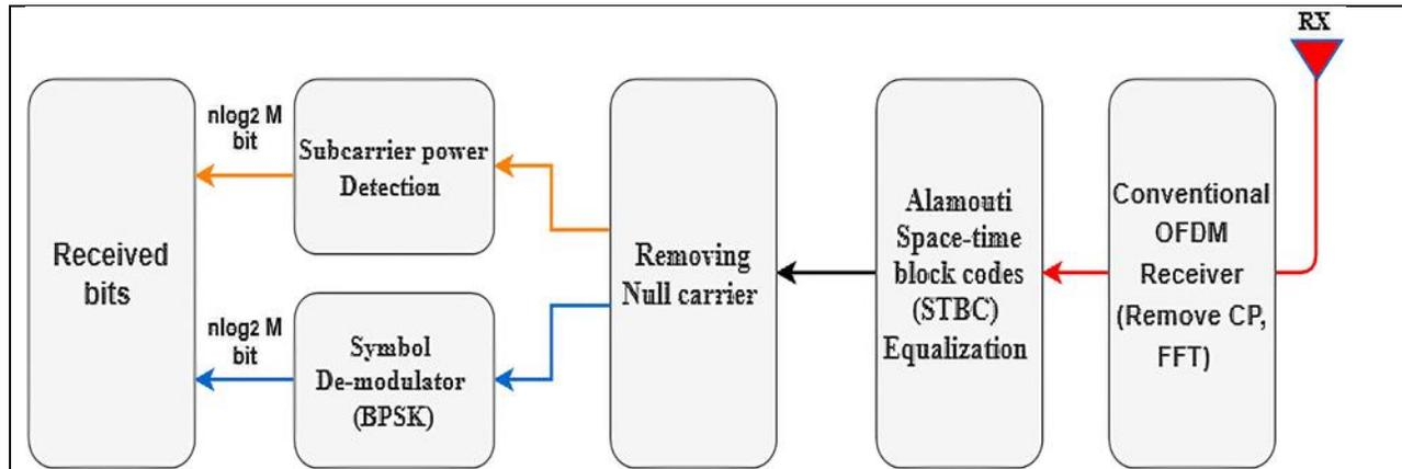
FIGURE 2: Receiver Design of OFDM-SPM with Alamouti STBC.
