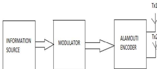
Figure 4: Alamouti space-time encoder diagram
