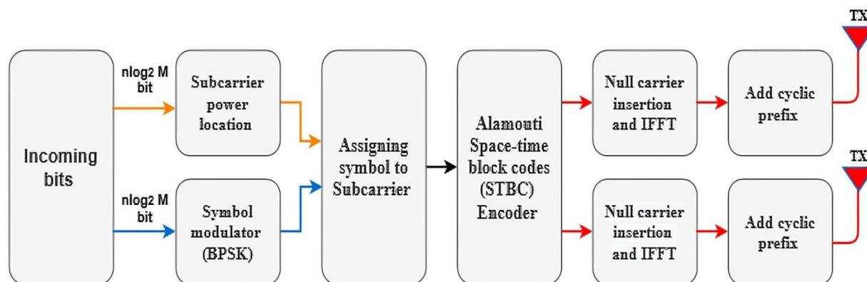
FIGURE 1: Transmitter design of OFDM-SPM with ALAMOUTI STBC
