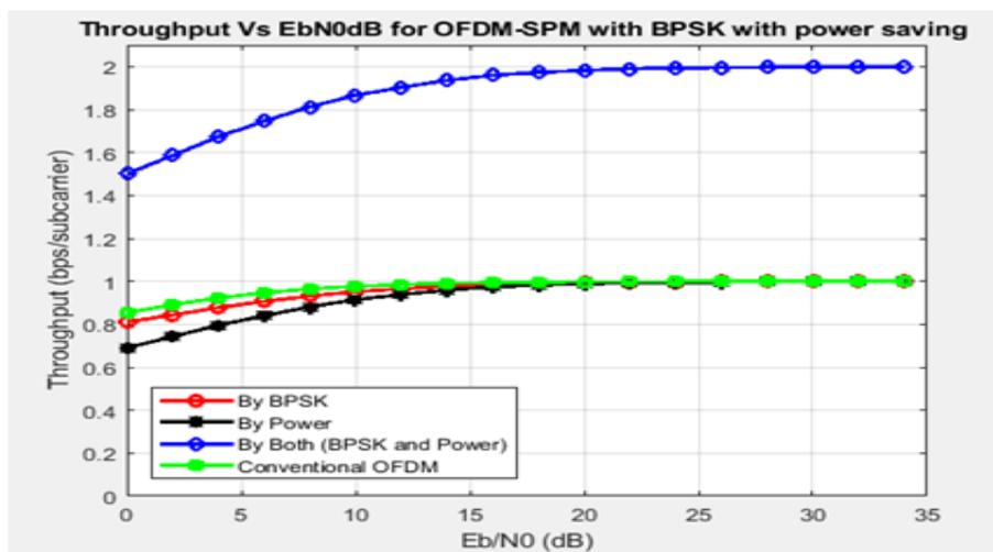
FIGURE 9: Throughput comparison for the proposedOFDM-SPM-BPSK-STBC
