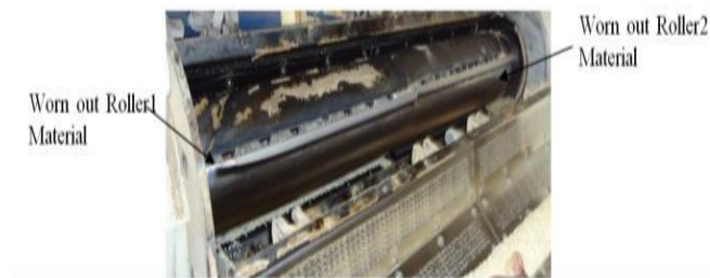
Figure 1: Rice Polisher Roller 1&2 Worn Out Condition
