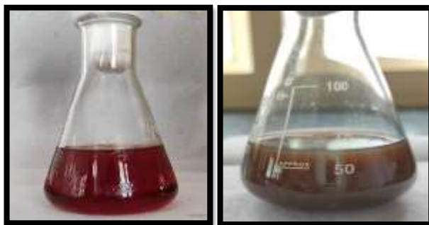
Fig 1: The colour change in the synthesis of copper nanoparticles.
