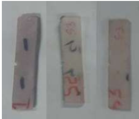
2(a) Before impact test specimen
