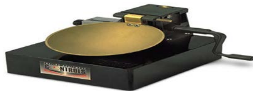
Figure 3 Liquid Limit experiment performed on Cassangrande apparatus
