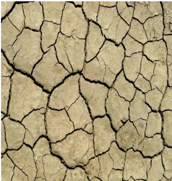
Figure 1. Cracks Developed in clayey soil ( after drying )
