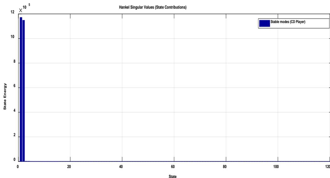
Fig.5 Bar chart of Hankel Singular Value of 120<sup>th</sup> Order Original System
