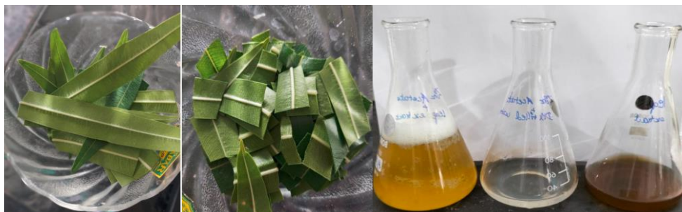
Figures 2, Mature leaves, Leaves in small pieces, Zinc Nitrate solution, aqueous extract of leaves and the mixture.
