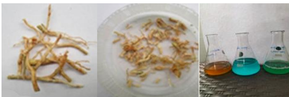
Figures 4. Root cuttings; Zinc Nitrate solution, aqueous extract of roots and the mixture.
