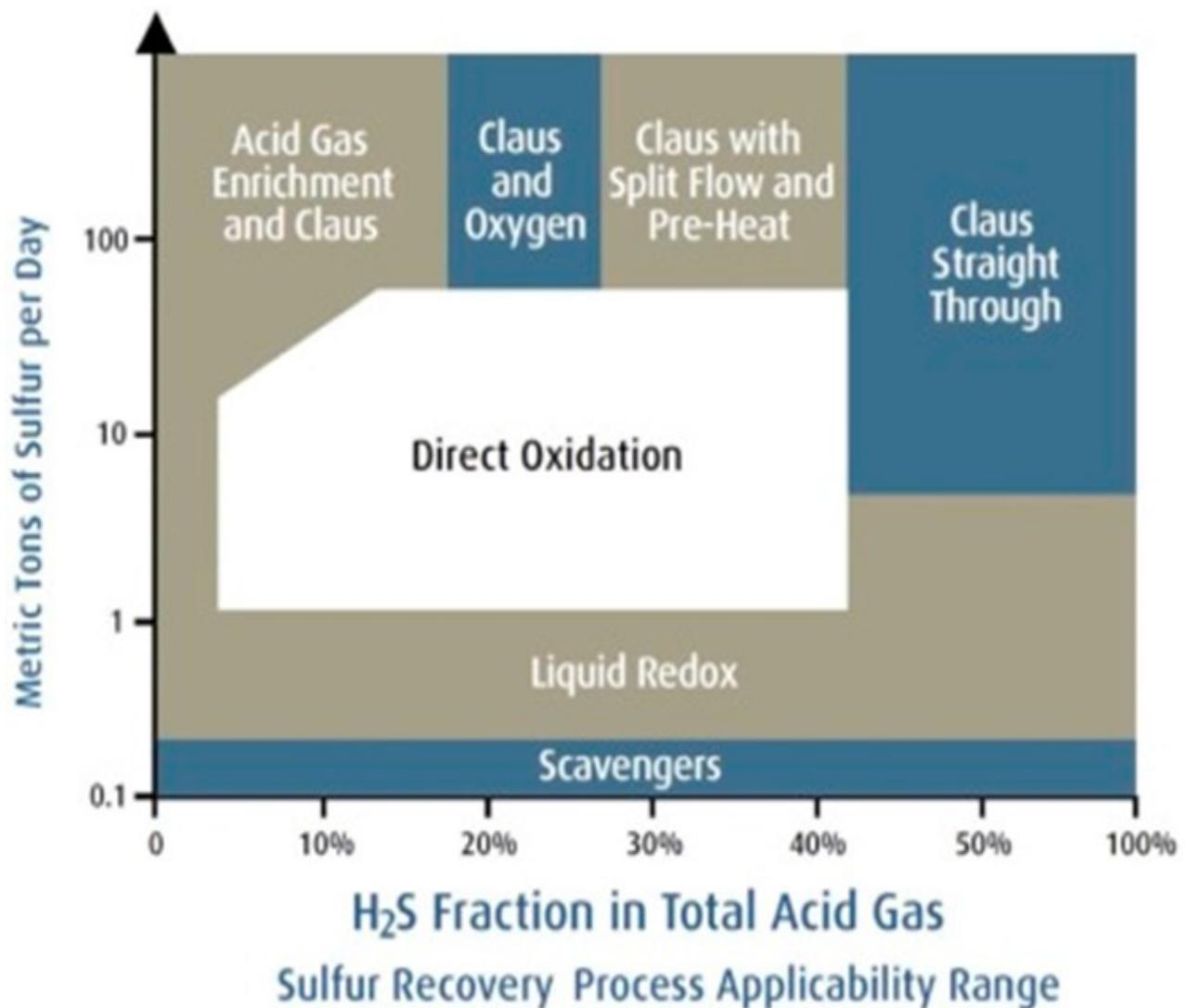
**Figure (1): Sulfur Recovery process Applicability Range**
