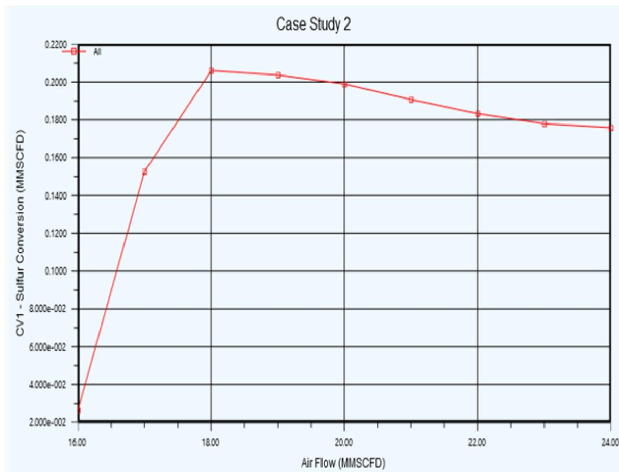
**Fig (7): The Effect of Oxygen Flowrate**
