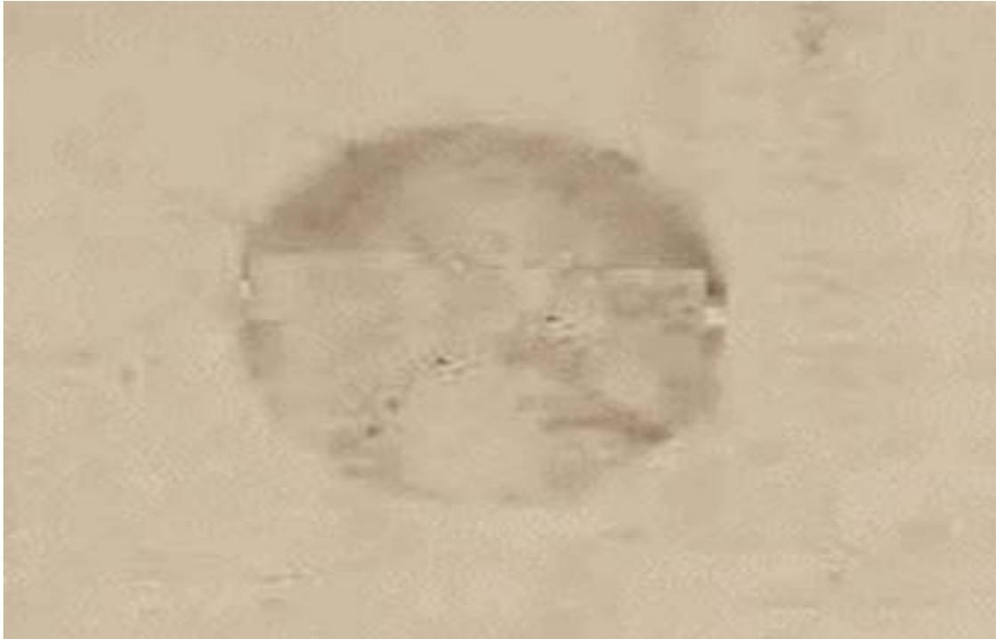
Fig 20: Optical images of the electrodeposited-calcined sample after Tape Adhesion test
