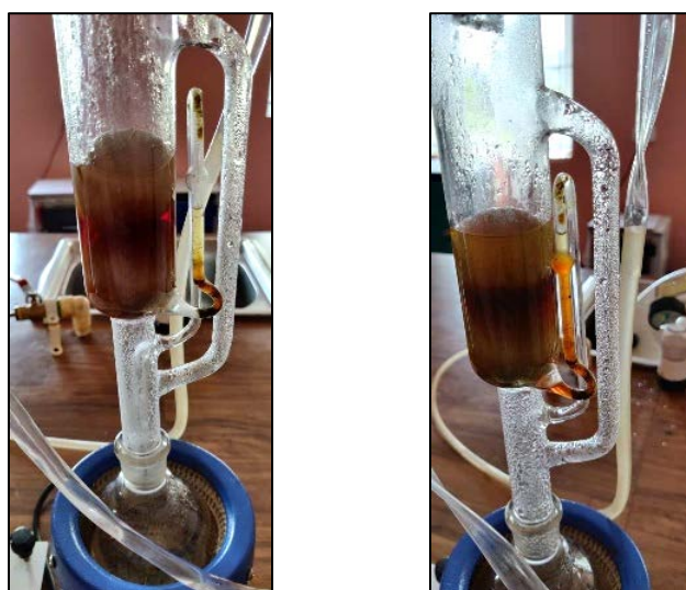
Fig. 2: Soxhlet apparatus and obtained solvent extracts stored in screw cap bottles
