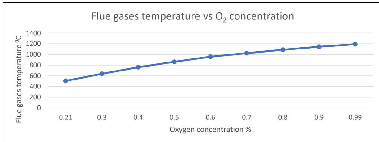
**Figure 6. relation between oxygen concentration and flue gases temperature**
