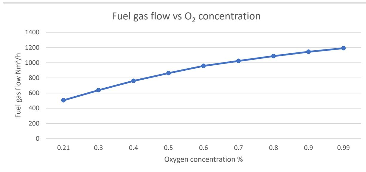
**Figure 4. relation between oxygen concentration and fuel gas flow**
