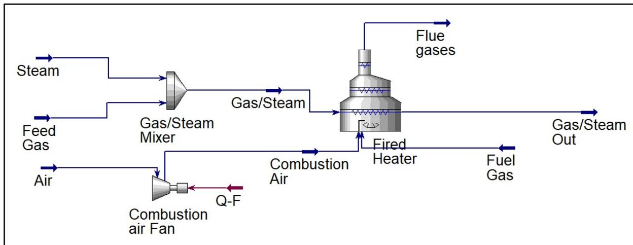
Figure 1. ASPEN HYSYS based Simulation of Process
