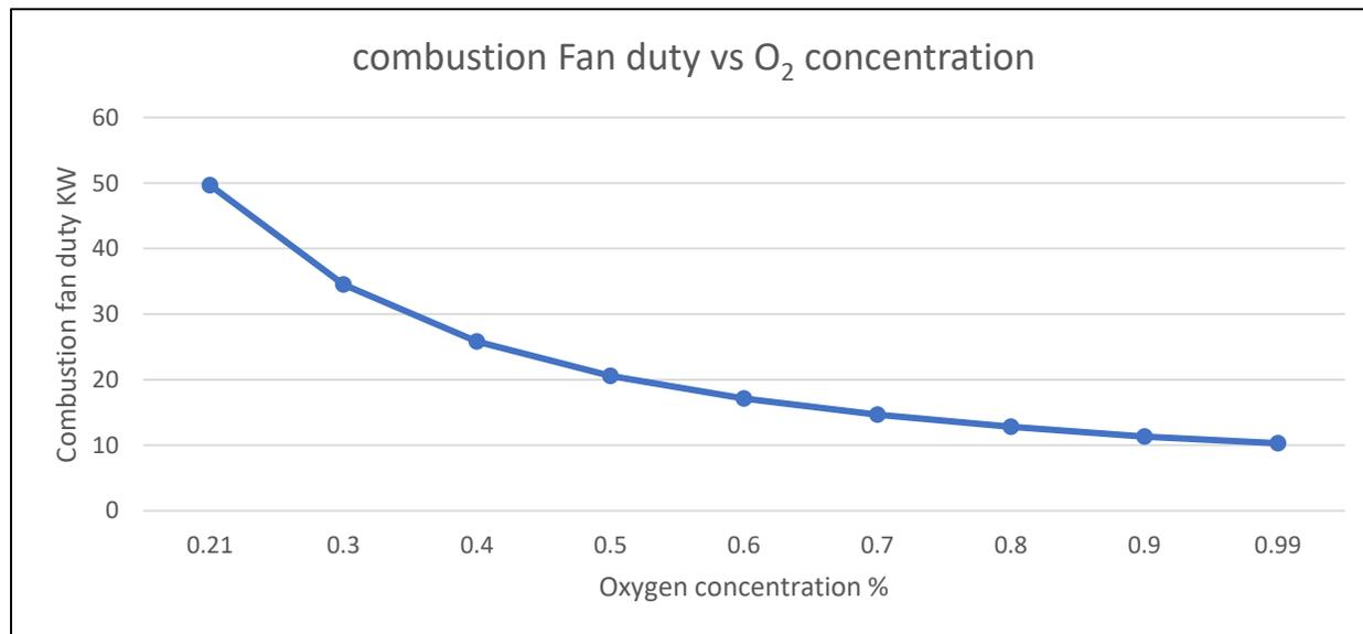
**Figure 3. relation between oxygen concentration and duty of combustion air fan**
