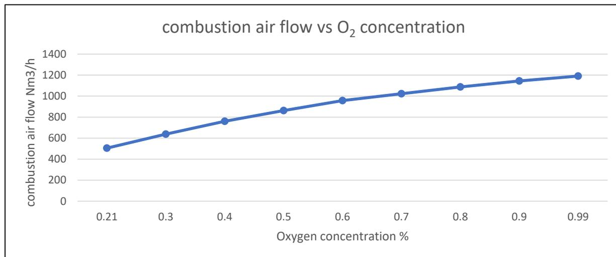
**Figure 5. relation between oxygen concentration and combustion air flow**
