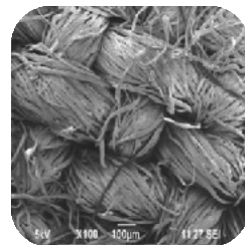
Fig. 2A: SEM analysis of Vetiveria zizanioides finished fabric sample under different magnification
