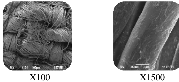
Fig. 3B: SEM analysis of Phyllanthusniruri finished fabric sample (Plasma treated) under different magnification
