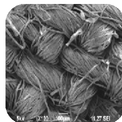
Fig. 2B: SEM analysis of Vetiveriazizanioides finished fabric sample (Plasma treated) under different magnification
