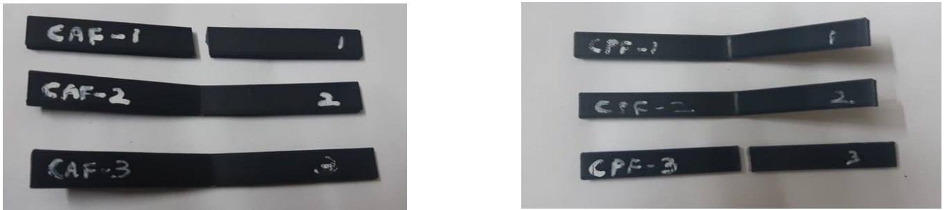
Figure.5. Comparative Analysis of Tensile Specimens Post-Failure: ABS versus PLA with Carbon Fiber
