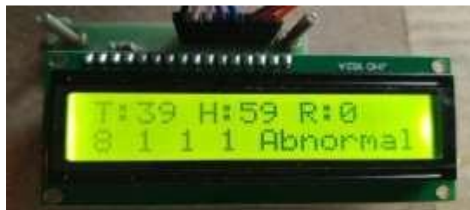
Fig.10. When LDR1 have higher intensity compared to other LDR's
