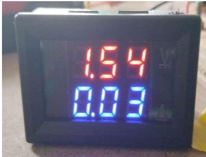
Fig.14. Device to shows the Output Voltage and current produced by Solar panel
