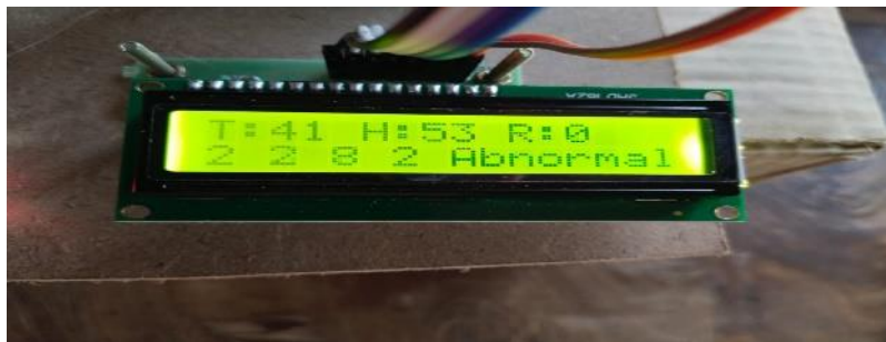
Fig.7. The readings of Temperature and Humidity displayed on LCD
