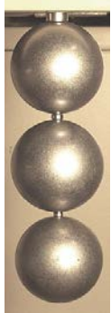
Neodymium magnets (small cylinders) lifting steel spheres. Such magnets can lift thousands of times their own weight.
