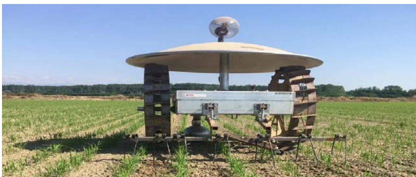
Figure 2: Autonomous paddy weeding robot [11] [Courtesy: www.futurefarming.com ]
