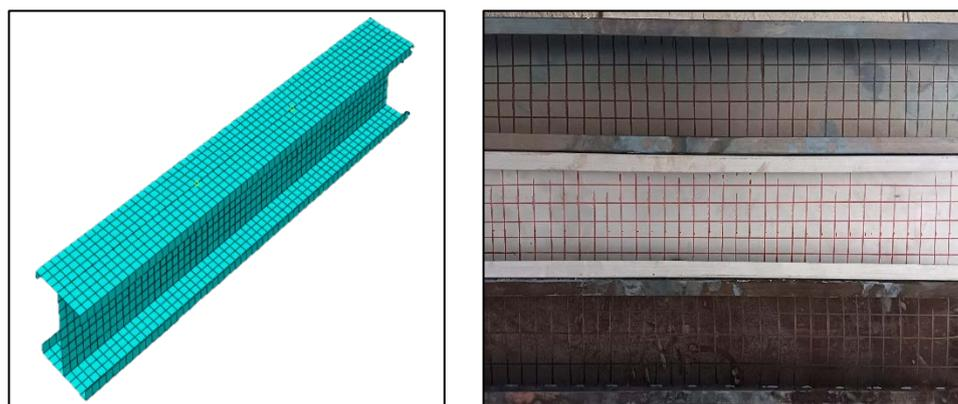
Fig. 4 Meshing on specimens a) FEM b) Experimental
