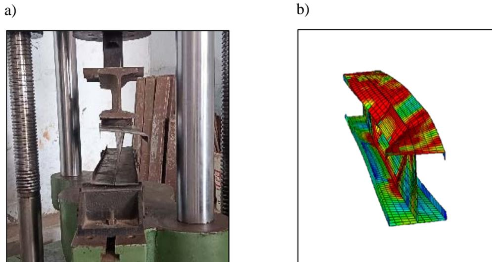
Fig. 7 Comparison of experimental and numerical behaviour at failure for specimen. a) Experimental and b) Numerical
