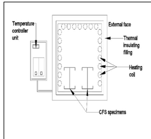
Fig.3 Beams in furnace.
