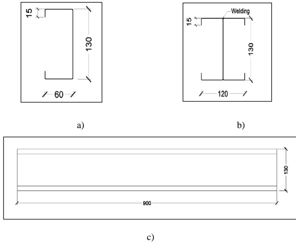
Fig. 1 Section geometry of built-up sections (a) Single channel section (b) Built-up 'I' section (c) Sectional view of the specimen.
