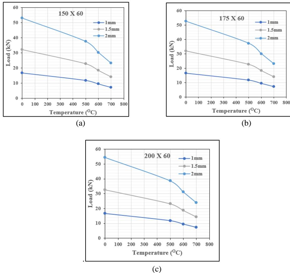
Fig.8 a) Load-carrying capacity of section 150 X 60. b) Load-carrying capacity of section 175 X 60. c) Load-carrying capacity of section 200 X 60.
