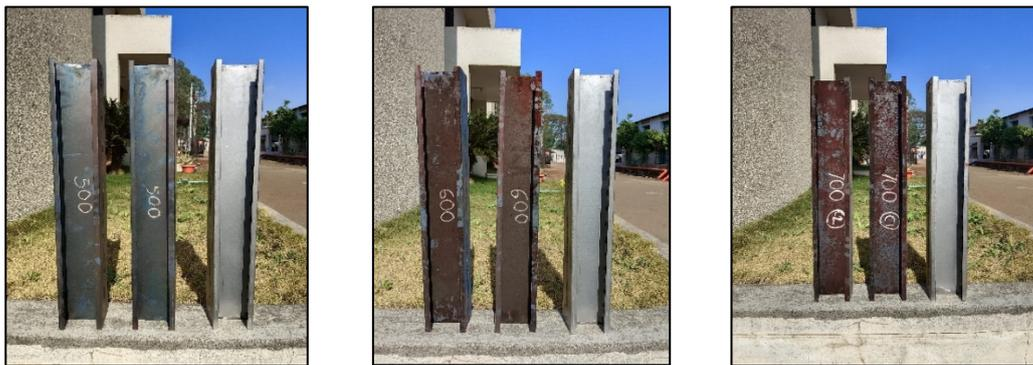
Fig.6 Colour change of 500°C, 600°C, and 700°C specimen.
