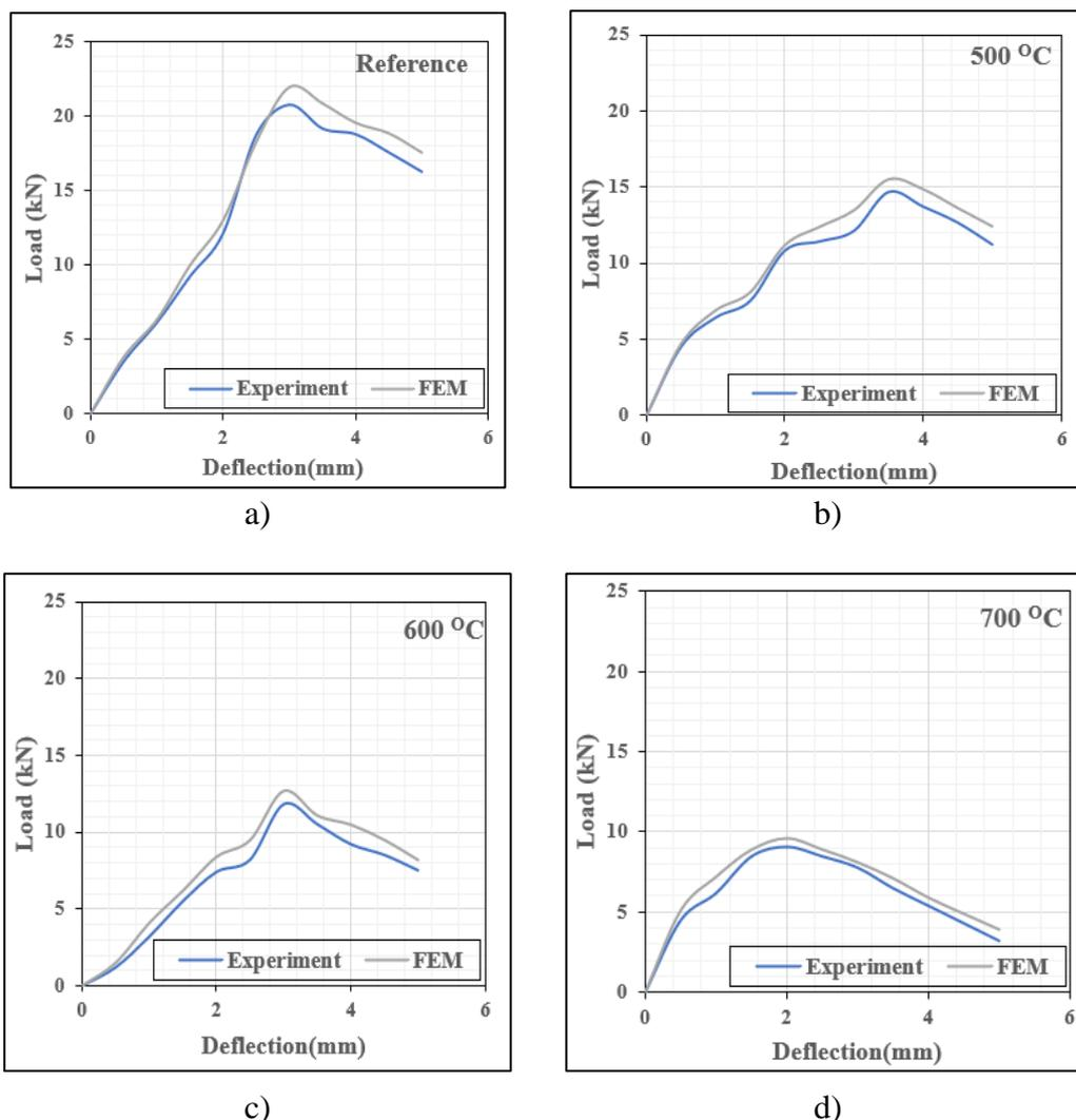
Fig.5 Comparison of Load vs Deflection for experiment and FEM of flexural behaviour specimens.
