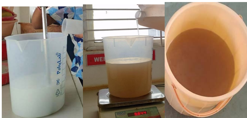
Figure: a)Preparation of NaOH, b) Sodium Silicate Solution, c) Alkaline Liquid
