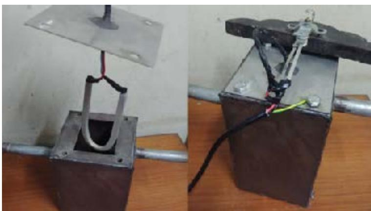
Figure 6. Assembled prototype heating system for evaporator setup
