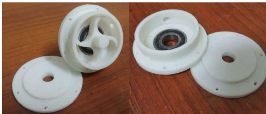
Figure 5. Designed Impulse turbine
