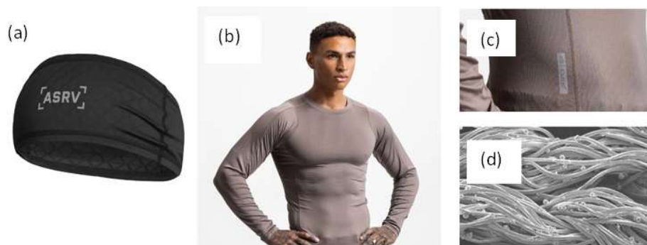
Figure 10: Phase change materials in sportswear maintaining microclimate (a) Outlast® incorporated headband by ASRV, (b) Outlast® incorporated full-sleeve by ASRV, [(c), (d)] textile coated with Outlast® utilizing MIC method.
